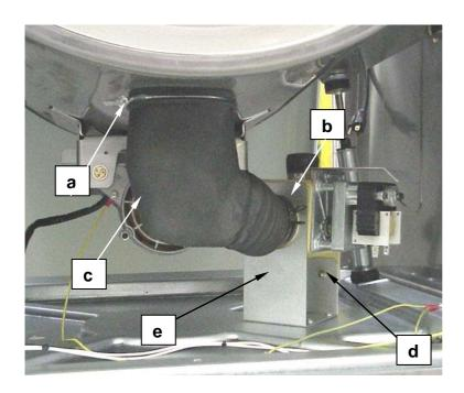
Loosen clamps (a, b) and remove the outer drum bellows outlet (c). Disassemble the screws from the support valve (d) and remove it. Remove the support (e) from the valve of the base of the machine.
