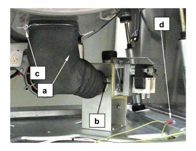
Mount the outlet bellows (a). Fasten it with the clamps (b, c). Fasten the ground cables with the screw (d). (In some machines, there is only one ground wire).
