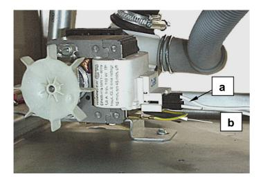
Disconnect electrical supply wiring (a) and ground wire (b) to the pump
