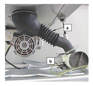
Remove the drain bellows (a) from the outer drum outlet and remove the support (b) of the pump from the base of the machine.
