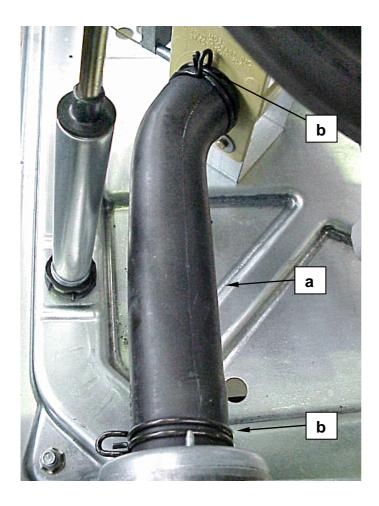
Mount the exit pipe of the valve (a) and fasten it with the clamps (b). Verify that the entire base of the washer is dry, with no water remaining.
