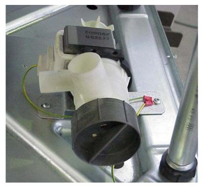
Fasten the pump assembly to the base of the machine.
