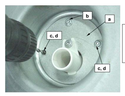
Position the supplement set + sleeve (a) over the lower rear cover and fasten it using screw b.
