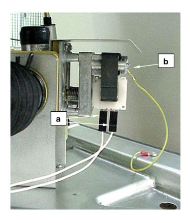
Disconnect electrical supply wiring (a) and ground wire (b).
