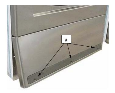
Open the lower front cover, removing the three screws (a) fastening the base and separating it from the machine.
