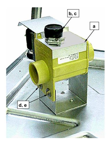
Position the protector plate (a) of the drain.
