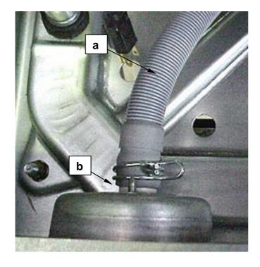
Remove the pipe (a) coming from the drain pump from the inside end (b) of the sleeve.
