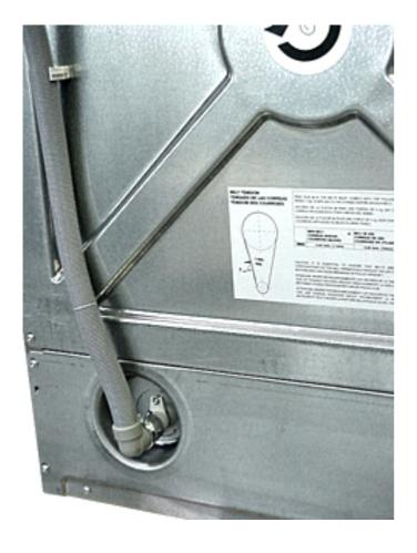
Remove the exterior drain pipe.
