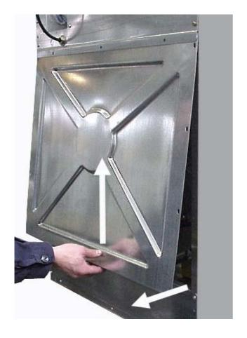
Open the central rear cover. Disassemble the fastening screws, moving the cover towards the top and separating it from the machine.
