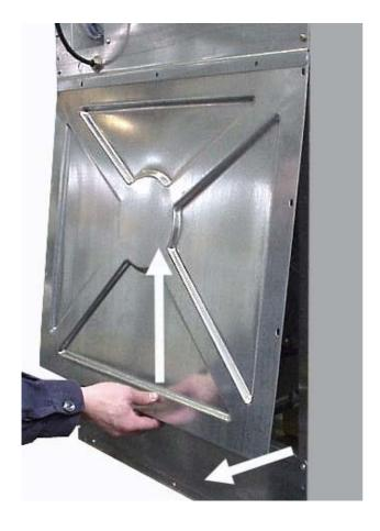
Open the central rear cover. Disassemble the fastening screws, moving the cover towards the top and separating it from the machine.
