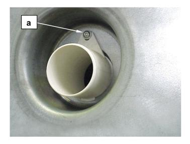
Remove screw **a**. Remove the sleeve from lower cover.
