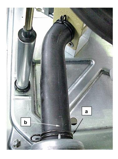
Remove the clamp (a) from the drain outlet pipe and separate the rear end of the pipe (b) from the drain sleeve.
