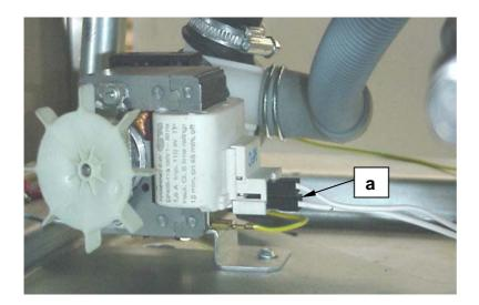
Connect the cables (a) of the electrical supply to the pump (there is no defined position for the connection of the cables)
