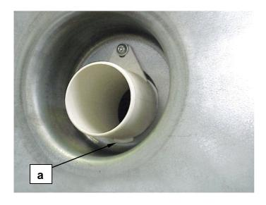
Mount the drain sleeve to the lower rear cover
