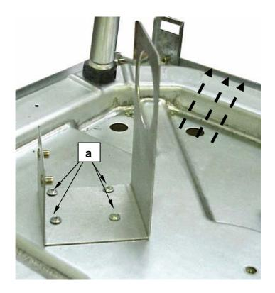
Mount the support of the drain to the base of the washer.
