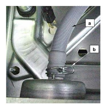
Insert the pipe (a) coming from the drain pump into the end of the hose and fasten it with the bracket (b)
